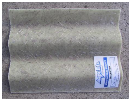
MELINEX 301 SHEET 8 YEARS NORTH FACING EXPOSURE SURFACE ERODED AND FIBRES EXPOSED
