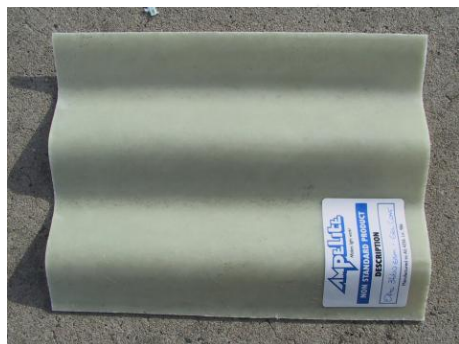
WONDERGLAS GC SHEET, 8 YEARS NORTH FACING EXPOSURE, SURFACE SMOOTH SURFACE INTACT, NO FIBRE SHOW
